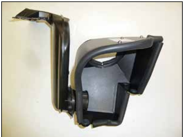
12. Install the factory fresh air intake scoop into the AEM® heat shield as shown.
