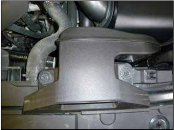
20. Install the factory fresh air scoop bolts.
