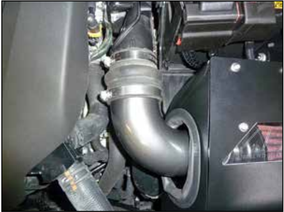
19. Install the intake tube into the coupler hose, adjust the tube for best fit and then secure the hose clamp.
