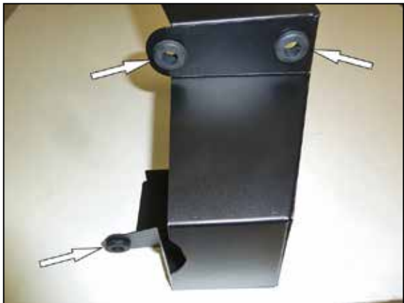
7. Install the three provided grommets into the heat shield as shown.
