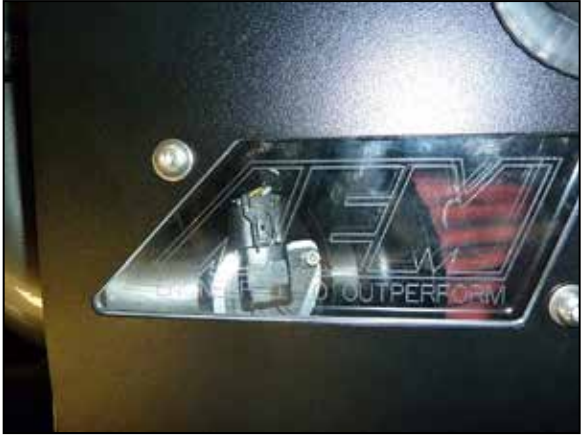
18. Reconnect the mass air sensor electrical connection.
