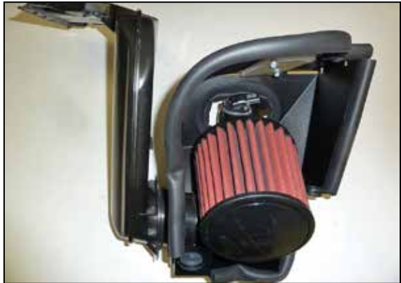
15. Install the intake tube assembly through the hole in the heat shield as shown.
