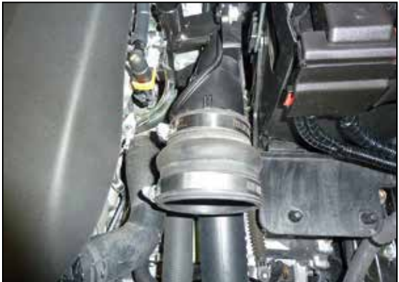
16. Install the hump coupler (5-574) onto the turbo inlet pipe and secure with the provided hose clamp.
